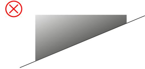
We're unable to do planterline panels with a sloped bottom edge.
