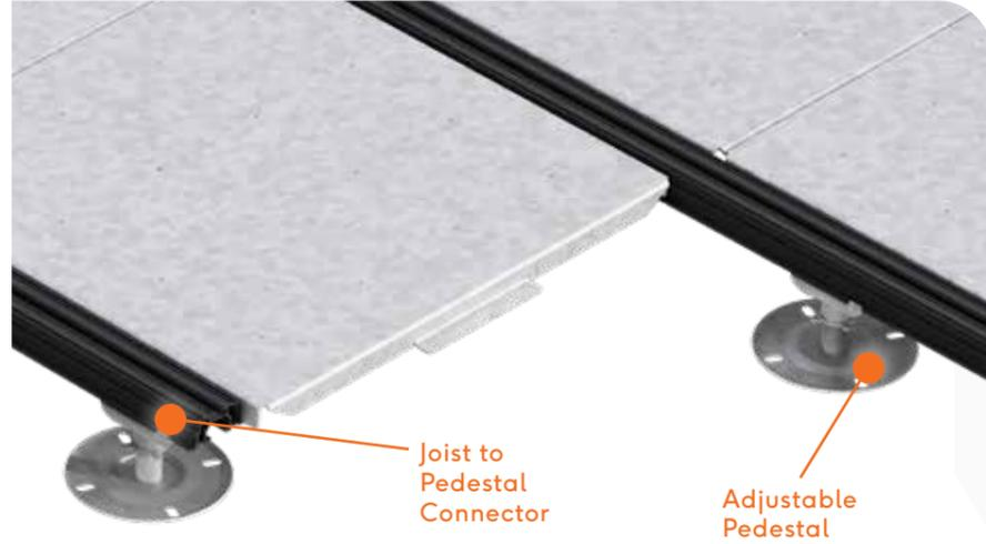
Rigid aluminium extruded joist rails for use as a support structure system to decking and paving. Raaft® joists are designed to be used on roof terraces, balconies and other external podium construction areas.
