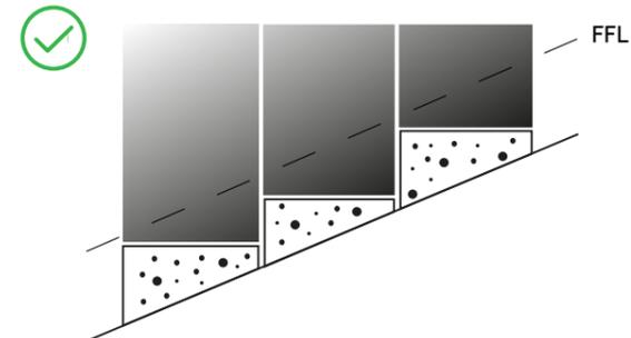
We can create level planters on a slope by stepping the concrete foundation and then changing the height of each planter panel to suit.
